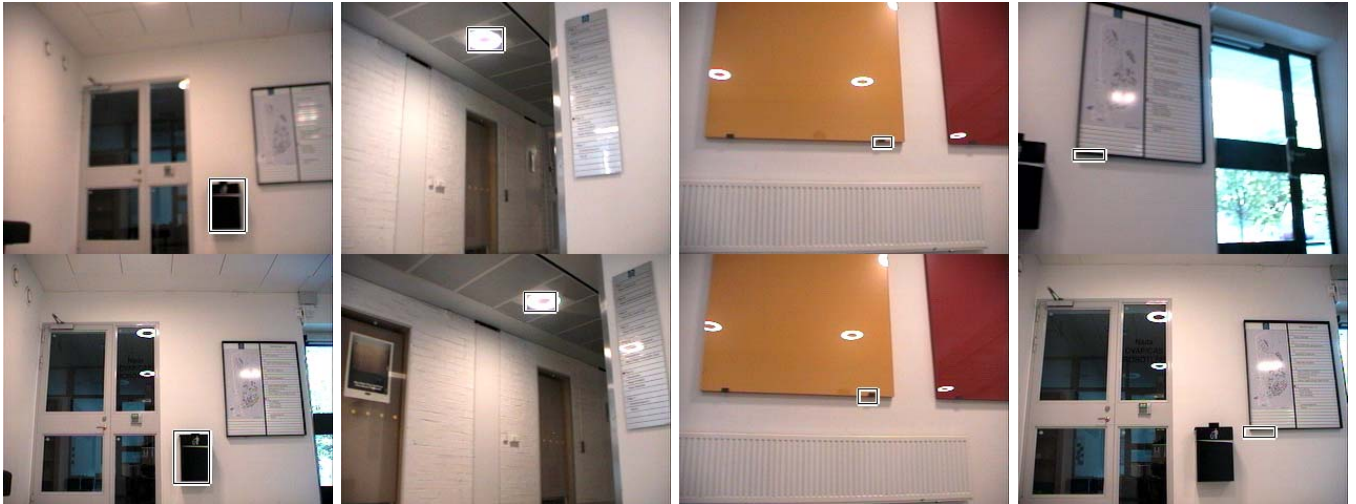
Fig. 9. Correct matches in loop closing situations: the first row shows a ROI in a current frame, the second row shows a previously stored ROI the current ROI was matched with. This situation usually occurred after the robot drove a circle and revisited the same area again.
