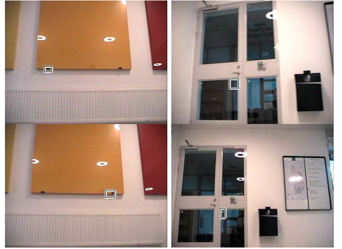
Fig. 10. False matches in loop closing situations: the first row shows a ROI in a current frame, the second row shows a previously stored ROI the current ROI was matched with. The matched regions are associated wrongly since they are highly ambiguous.
