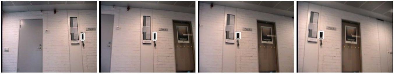
Fig. 8. Tracking of a landmark after 1, 10, 15, 20 frames with \delta = 5.0 and additional position prediction.
