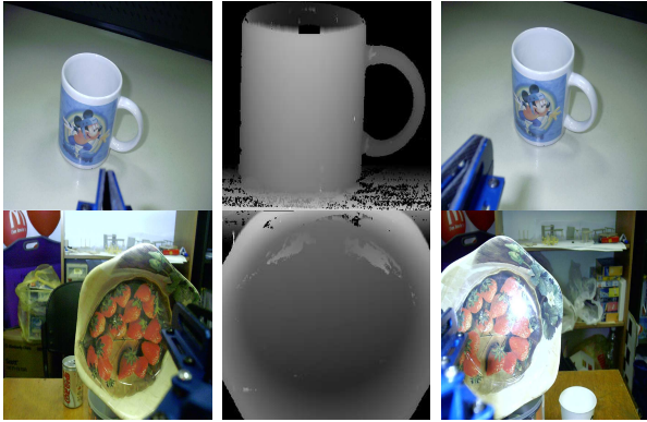
Fig. 3. On each row, left and right images as taken from the robotic arm in Figure 4. The middle images are their range reconstruction.
