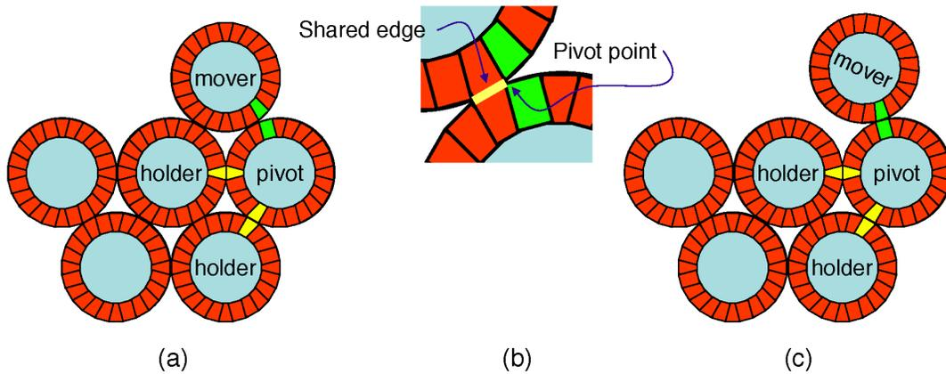
Fig. 2. A typical movement scenario. (a) is the start configuration. (b) is a blow up of the mover-pivot pair. (c) is the final configuration. The yellow magnets exert a small holding force. The green magnets exert a large force to move the mover around the pivot.
