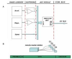
Fig. 4 A/D conversion and communication protocol: (A) logic diagram of A/D conversion; (B) communication protocol
