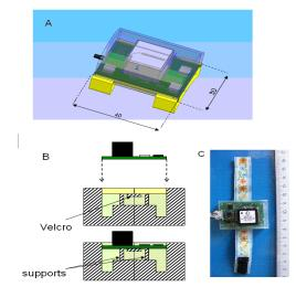
Fig. 3 Mechanical design: (A) First design; (B) ; Fabrication steps; (C) Final result: the silicon support structure embedding electronic board and Velcro straps.
