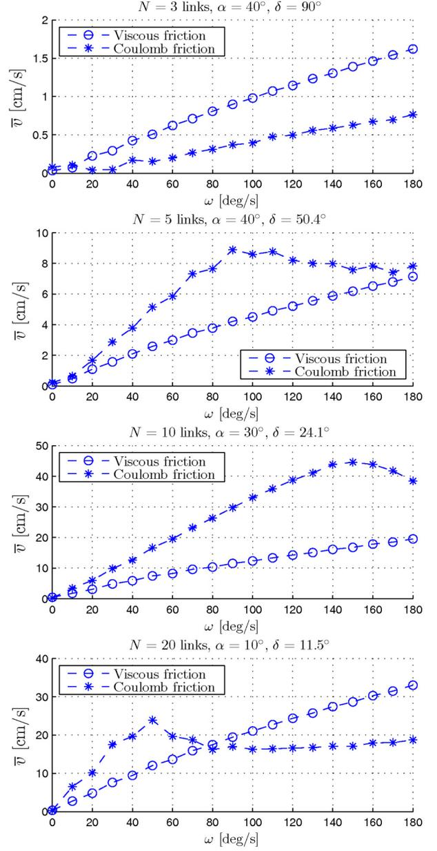
Fig. 8. The average forward velocity of the snake robot for different values of  $\omega$ . The number of links  $N$  and the corresponding values of  $\alpha$  and  $\delta$  are shown at the top of each plot.
