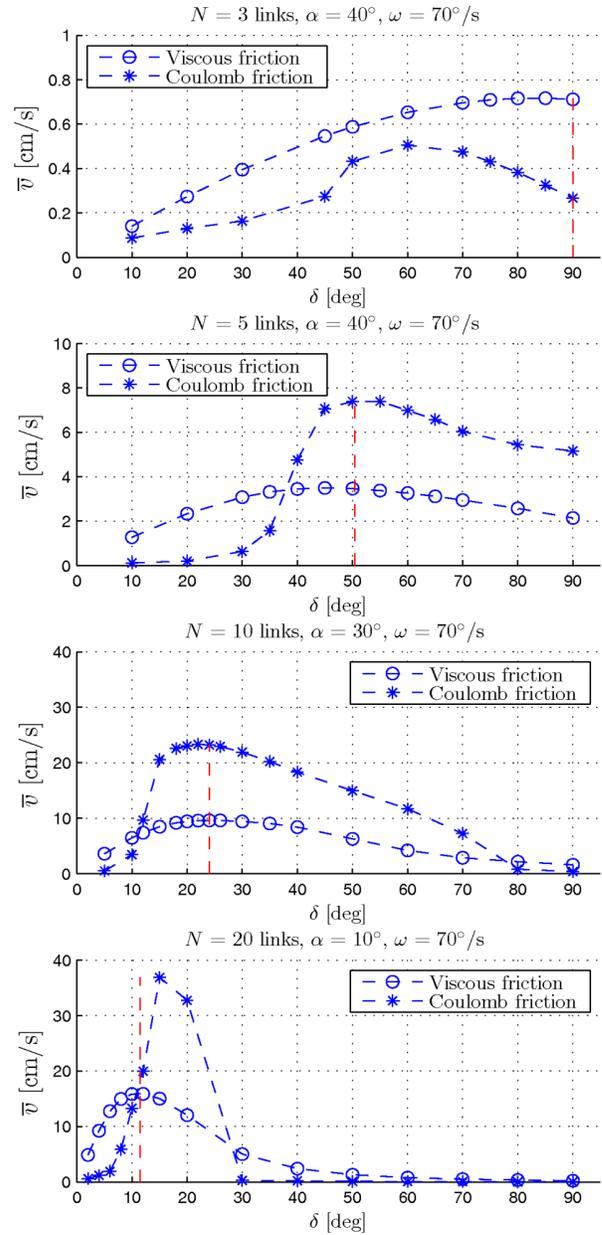
Fig. 10. The average forward velocity of the snake robot for different values of  $\delta$ . The number of links  $N$  and the corresponding values of  $\alpha$  and  $\omega$  are shown at the top of each plot.
