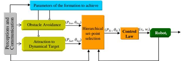
Fig. 2. The proposed architecture of control.
