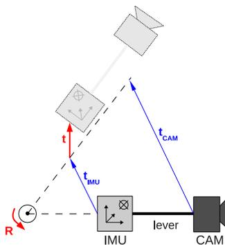
Fig. 1. The drawing sketches the motion of a camera-IMU setup. Both sensors measure the applied rotation ( $R$ ) and translation ( $t$ ). The only difference is the different lever action ( $t_{\text{IMU}}$ ,  $t_{\text{CAM}}$ ) due to the baseline introduced by the rotation.
