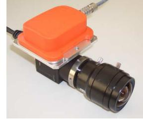
Fig. 3. A PointGrey Flea2G camera with wide angle lens and a Xsens-MTi IMU (orange box) as it is used in our experiments.
