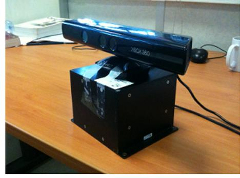
Fig. 3. Kinect mounted on an IMU
