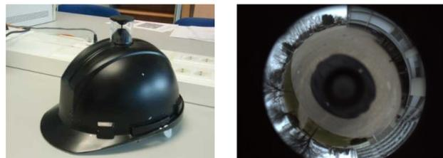
Fig. 1: (a) Hemlet-camera device used in our experiments. (b) Omnidirectional image captured with our device.
