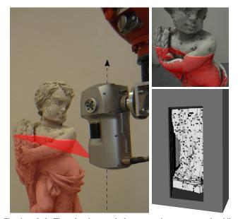
Fig. 1. *Left:* The robot is moved along a continuous scan path while the statue is scanned with the attached laser stripe profiler. *Upper Right:* A triangle mesh is reconstructed in a real-time stream during the sensor movement. *Lower Right:* The initially unknown space (gray) is updated based on sensor data of the current scan.
