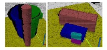
Fig. 9. Left: The bin is separated caused by planar model applied to curved surface. Right: Small box splitted due to wrong order of split faces.
