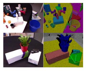
Fig. 8. Top: A complex scene with multiple support planes and nonconvex objects. Bottom: A scene with a complex object (plant), segmented model-free and without previous knowledge about this object
