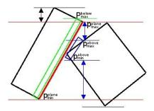
Fig. 5. Assigning separating plane using bounding boxes.
