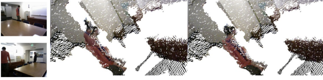
Fig. 3. Left: When a naive nearest-neighbor metric is applied, two sides of an object will be drawn toward each other, often at the expense of violating free space. Right: Our occlusion-aware energy term is able to recover from many of these situations.
