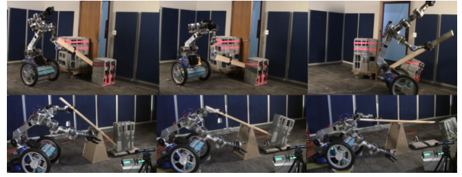
Fig. 9. Key motion steps in pushing and overturning heavy objects
