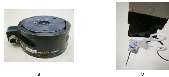
Figure 3: The experimental setup. a) Force/torque sensor, b) PUMA robot, equipped with a laparoscopic surgical tool.
