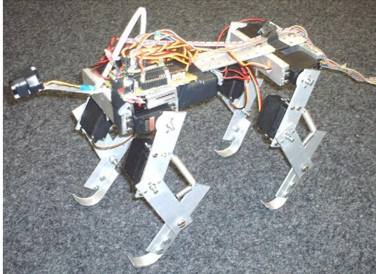
**Figure 2.3.:** Elastic four-legged robot Puppy
