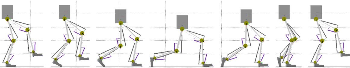
**Figure 8.17.:** The sequence shows the robot motion with the optimal configuration of active and passive control parameters for walking (configuration number 4 in Tables 8.12 and 8.14).
