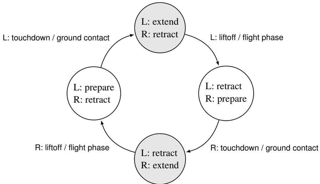
**Figure 8.14.:** The graph displays the structure of the state machine, which is applied in the present example. Overall there are four states, which are triggered by the flight phase or contact phase of either of the two feet. The state machine returns the respective target motor position for all involved joints (hip, knee, and ankle) for both legs.
