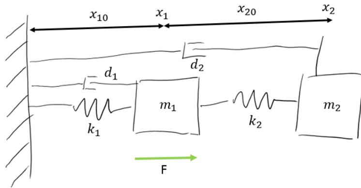
**Figure 8.1.:** The image shows a sketch of the setup for the swinging mass example. Involved parameters are the masses  $m_1$ ,  $m_2$ , the spring coefficients  $k_1$ ,  $k_2$ , the damping coefficients  $d_1$ ,  $d_2$ , the equilibrium lengths  $x_{10}$ ,  $x_{20}$ , the equilibrium positions  $x_1$ ,  $x_2$ , and the applied force  $F$ . Although the image depicts a spacial expansion of the involved masses, they are considered as point masses.
