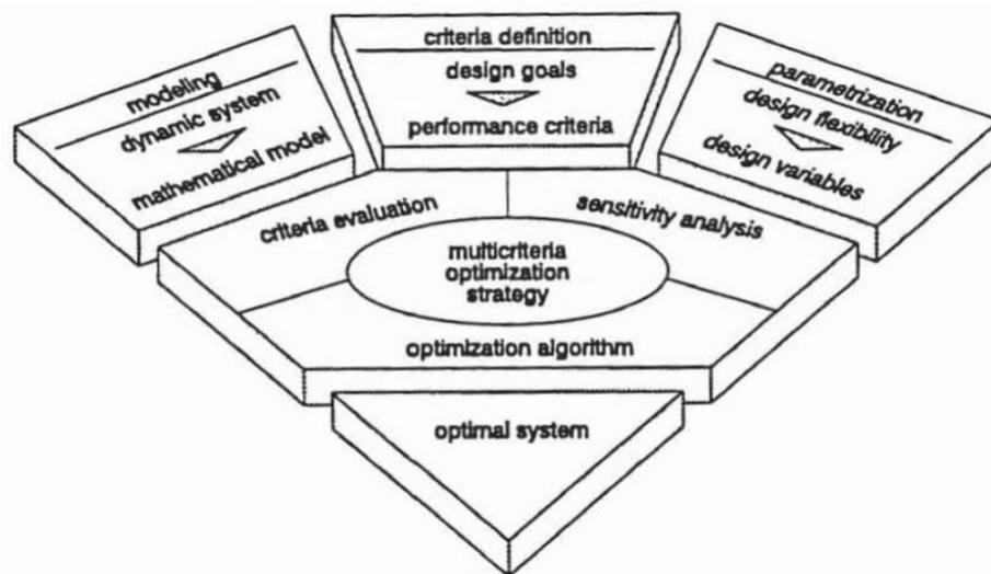
**Figure 2.5.:** Components of an optimization-based development approach
