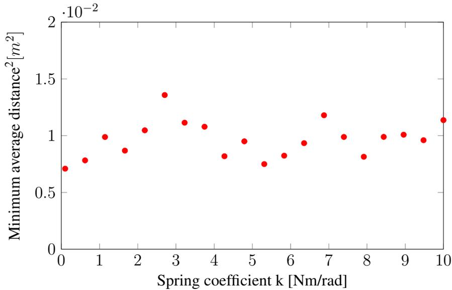
**Figure 8.8.:** In this plot the optimal result for each considered spring coefficient is depicted regarding the simulation experiment to optimize robustness. Each result represents the minimum quadratic average distance to the target position with respect to the involved set of perturbations.
