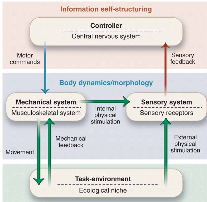
**Figure 2.2.:** The fact of being embodied implies instantaneous feedback of the task-environment to the morphology of the system resulting from interactions with the environment. The layer of body dynamics also includes the reception of sensor stimuli with respect to the morphology. In a higher level control layer the sensor signals are processed and (feed-forward) motor commands are generated.
