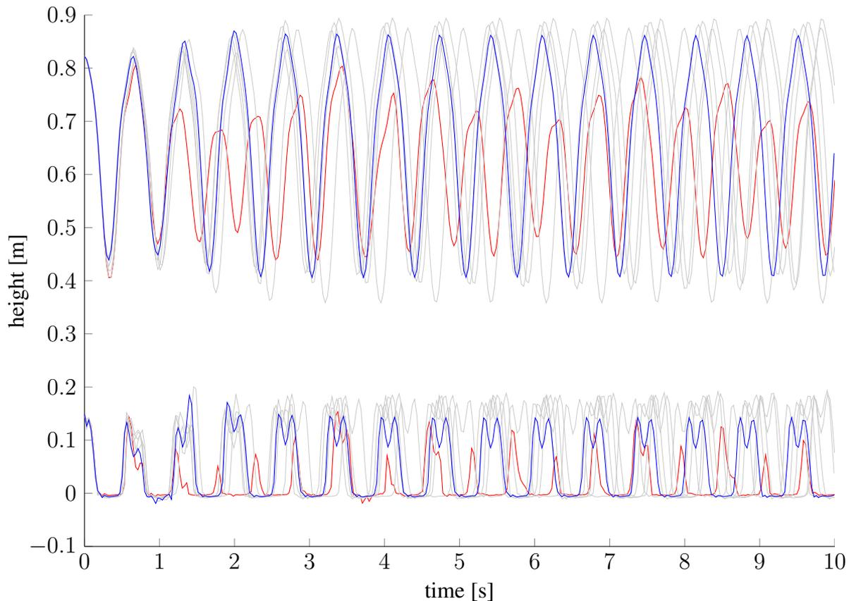
**Figure 8.13.:** Hopping trajectories of the Pareto-optimal solutions of the 1D hopping example. The upper trajectory depicts the position of the hip joint over time and the lower trajectory the position of the foot-tip. The optimal trajectory when only considering problem formulation 1 is depicted in blue, while the optimal solution when only considering problem formulation 2 is depicted in red. Further Pareto-optimal solutions are shown in grey.
