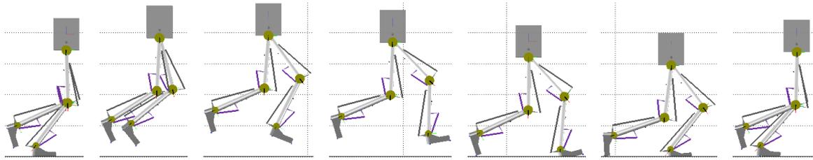
**Figure 8.16.:** The sequence shows the robot motion with the optimal configuration of active and passive control parameters for jogging (configuration number 1 in Tables 8.12 and 8.13).
