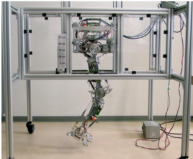
**Figure 8.11.:** The BioBiped 2 robot is constrained to a single translational DOF by the supporting frame.
