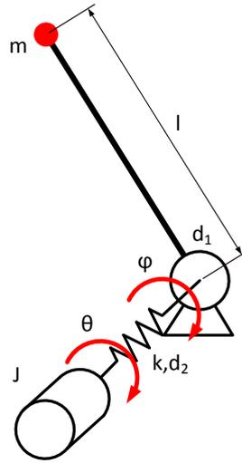
**Figure 8.7.:** 3D-schematic of the considered robotic arm with one DOF. The actuator with Inertia  $J$  and motor angle  $\theta$  shown in front is connected to the arm via an elastic element. The elastic element has a spring coefficient  $k$ , and damping  $d_2$ . The arm itself has a joint damping  $d_1$ , length  $l$  and the point mass  $m$  on its end.  $\varphi$  describes the current angle of the arm. Zero positions for  $\theta$  and  $\varphi$  are in straight upward position.
