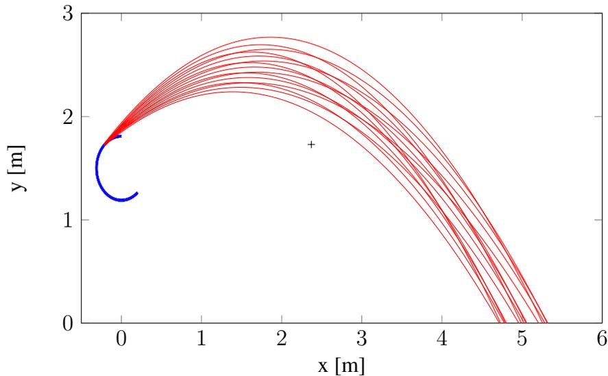
**Figure 8.10.:** The figure shows the set of trajectories which result from the optimal configuration with respect to the performance goal. The blue curves hereby depict the trajectory of the mass while in contact with the arm. The red curves depict the respective flight paths that result from the optimal configuration for the considered parameters and the applied set of perturbations. The black plus indicates the target of the robustness goal. It is displayed for convenience.
