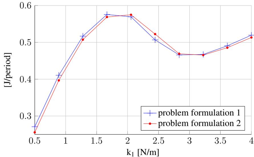
**Figure 8.5.:** Resulting minimal energy requirements for the desired motion regarding only the considered spring coefficients  $k_1$ . It must be considered, that only marked configurations are evaluated. Lines in-between are interpolated.
