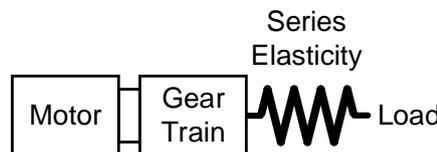
**Figure 4.2.:** The configuration of a series elastic actuator: Motor and gear train are connected via an elastic element to the respective load.
