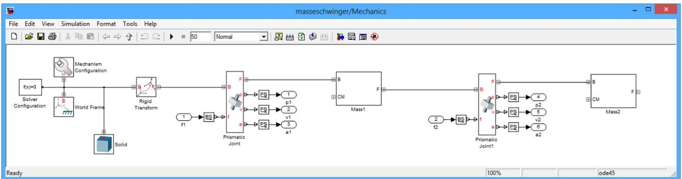
**Figure 8.3.:** The picture depicts an overview of the symbolic implementation of the dynamic behavior of the swinging mass in MATLAB® Simulink® SimMechanics™.
