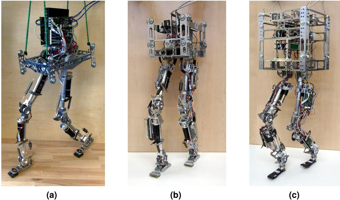
**Figure 6.1.:** The comparison of the three BioBiped generations (a) BioBiped1 from 2010, (b) BioBiped2 from 2012, and (c) BioBiped3 from 2014 reveals its phylogenetic evolution. Several details were enhanced based on experiences to enable a better achievement of the desired motion goals.
