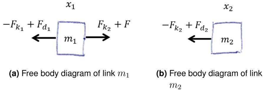
**Figure 8.2.:** The illustrations show the respective free body diagrams of the the involved links of the swinging mass example.
