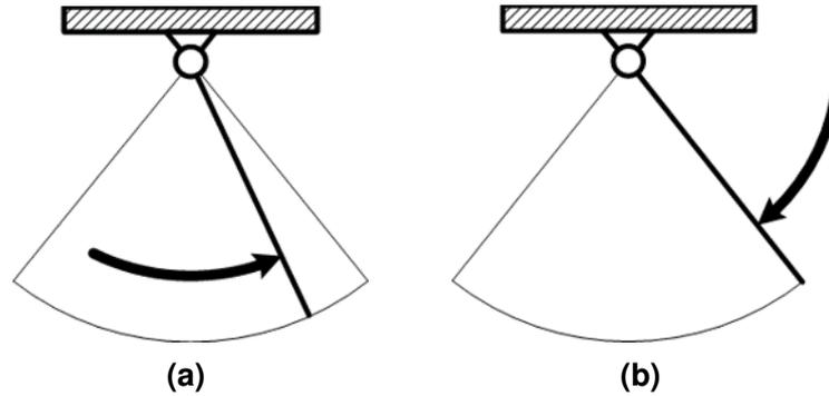
**Figure 3.2.:** “Expensive design”: The pendulum is actuated in the joint and desired to oscillate in the marked area. Without the exploitation of physical effects the operation is not “cheap”.
