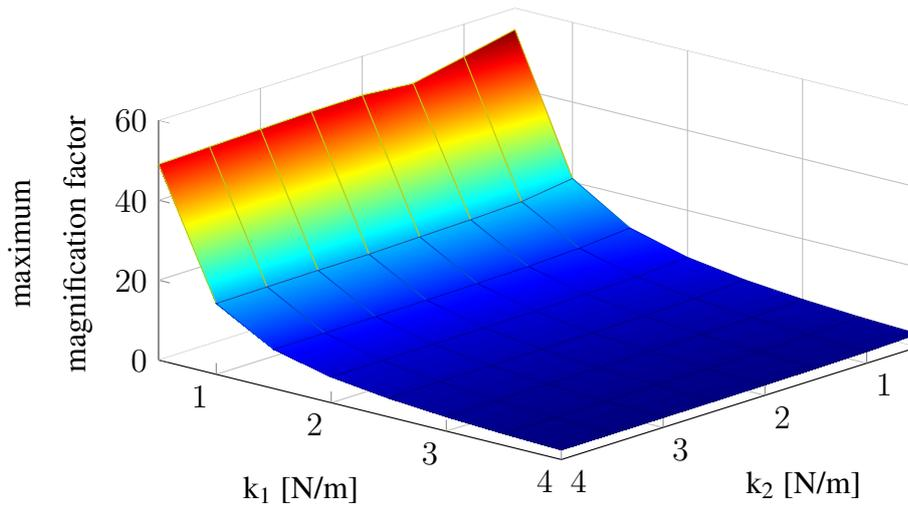
**Figure 8.6.:** Maximum magnification factor of each configuration  $[k_1, k_2]$  for problem formulation 1. The magnification factor is calculated with a simplified equation of motion. Problem formulation 2 results in a similar configuration.
