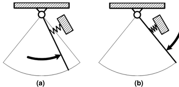
**Figure 3.3.:** “Cheap design”: By the application of a suitable elastic element the operation is supported. Less energy must be applied. Another obvious approach is the application of a torsional spring. The presented setup however is related to the examples presented in Sections 8.3 and 8.4
