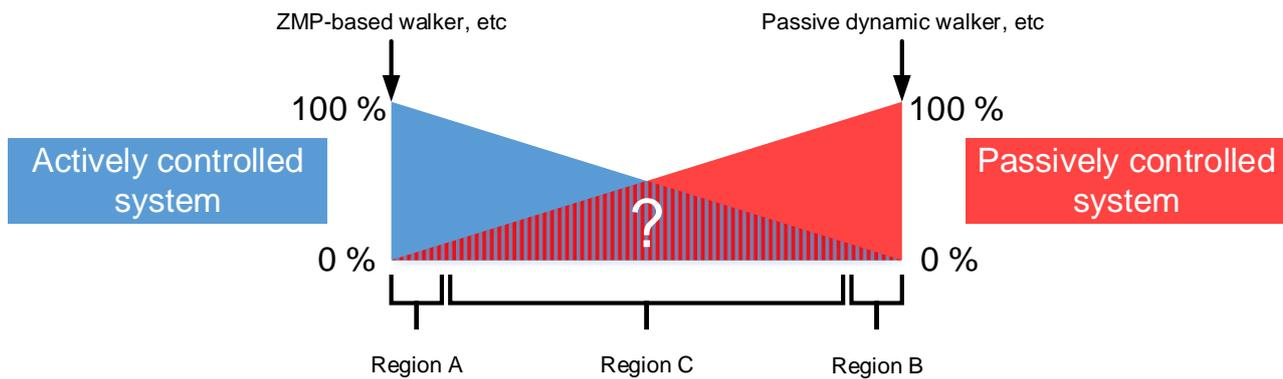
**Figure 2.1.:** A graphical representation of possible task distribution between control and mechanical systems in generating behavior. Most of the current robots are driven under the task distribution either around the left or right extremity. [41]
