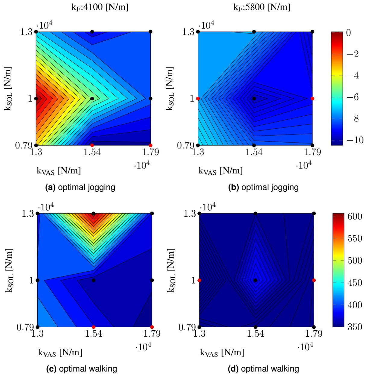
**Figure 8.15.:** These plots depict the optimal objective value for each considered spring configuration. Figures 8.15a and 8.15b show the optimal values for jogging, according to Equation (8.34). Figures 8.15c and 8.15d show the optimal objective values for walking, based on Equation (8.35). Evaluated configurations are marked with a black dot, while Pareto-optimal configurations are marked with a red dot.
