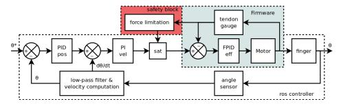
Fig. 1. Internal mixed position velocity controller with safety force limitation
