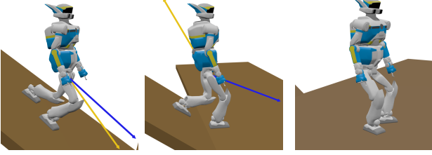
Fig. 7: Key captures of HRP-2 going down a 38° slope.
