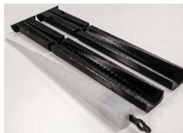
Fig. 3. Silicone based compliant arm and mold.
