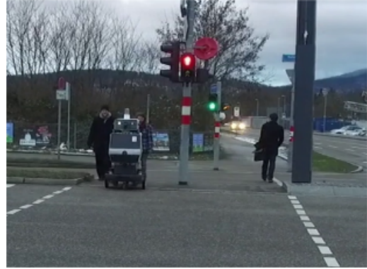
Fig. 1. Autonomous navigation at a street intersection by combining information from different modalities. The figure shows our robotic platform at a street intersection, where it uses the data from the laser and radar sensors to decide when it is safe to cross.
