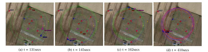
Fig. 3: Screenshots from the Paparazzi ground control station showing the evolution of the circular formation.
