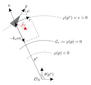
Fig. 1: The direction to be followed by the UAV at the point  $p^*$  for converging to  $C_r$  is given by  $\hat{p}_d$ . The tangent and normal vectors  $\tau$  and n are calculated from  $\nabla \varphi(p^*)$ . The error *distance* e is calculated as  $\varphi(p^*)$ . All the circles  $\varphi_c$  can be parametrized by an angle  $\theta$  with respect to the horizontal axis of a frame of coordinates at the center of  $C_r$ .
