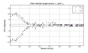
Fig. 4: Inter-vehicle error angle evolution. The zone  $\pm 10$  degrees is between the dashed lines. Each dot represents the calculated error by one of the airplanes once it receives the position of its neighbor. The density of points is different due to lost communications. However, the algorithm seems robust enough against such an issue as it drives both errors close to zero within a band  $\pm 10$  degrees.
