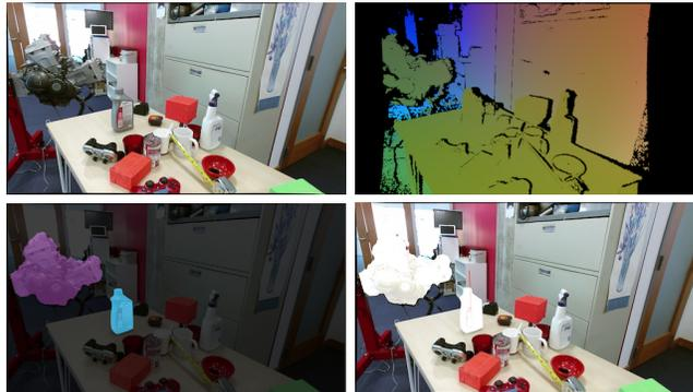
**Fig. 5: Automatic Motion Capture Annotation:** Given input RGB and encoded depth images (top row), the automatic labeling system outputs the segmentation and object poses in axis angle format (bottom row).
