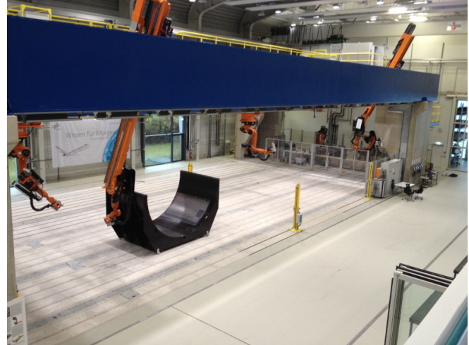
Fig. 1. Multifunctional robotic cell at the DLR Augsburg with ceiling mounted robots on linear tracks. On the shop floor a tooling of the lower fuselage of an Airbus A320 with two meter length has been positioned.
