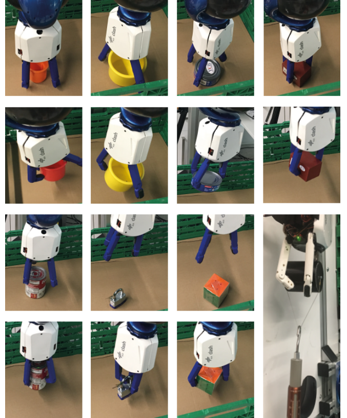
Fig. 16: Grasping household objects from the YCB object dataset. The lower-right picture shows a pull out test for a cylinder with diameter 60mm, resulting in a pullout force of 28N.
