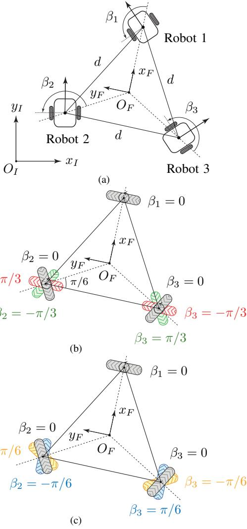
Fig. 3. Three unicycles. (a) Formation defined by three distance constraints; (b), (c) Special orientations of the m-wheels of the m-robot (for the sake of illustration, we set  $\beta_1 = 0$  in both cases).
