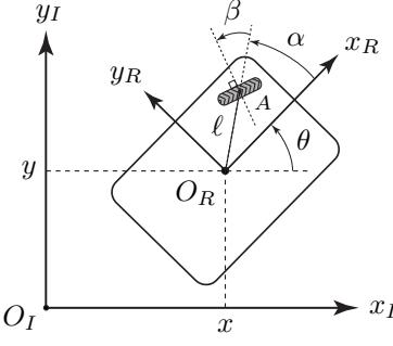
Fig. 1. Notation for a conventional centered wheel of a mobile robot.
