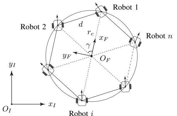
Fig. 4.  $n$  unicycles. The formation is specified by  $n$  distance constraints. The regular convex polygon has side  $d$  and circumradius  $r_c$ .
