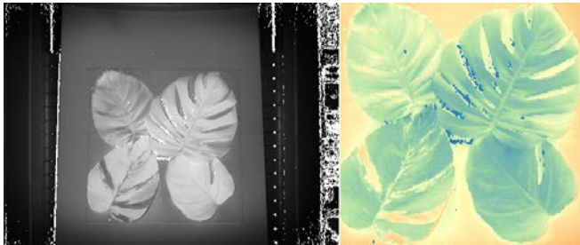
Figure 12. Left: NDVI greyscale generated image; Right: NDVI colored mapped image. Green color means high NDVI value
