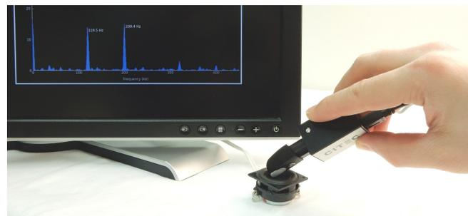
Fig. 7. The fingernail held against a computer controlled shaker (loud-speaker) generating a dual tone sinusoidal waveforms at 120 Hz and 200 Hz, while a live FFT of the accelerometer Z-axis signal is displayed on screen. The peaks are detected at the awaited frequencies.
