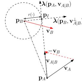
Fig. 7: Illustration for deriving  $d_{AB}^{CPA} = r(\mathbf{p}_B, \boldsymbol{\lambda}(\mathbf{p}_A, \mathbf{v}_{A|B}))$ .
