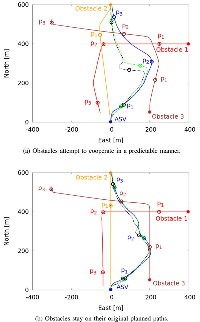
Fig. 6: Simulation of different behavior cases involving head-on, crossing and overtaking scenarios. Different behaviors are recorded for the ASV using DRVO (blue), RVO (green), and VO (black). The locations  $p_1$ ,  $p_2$ , and  $p_3$ , indicate the positions of the obstacles and the ASV at the same sampling time. In (b) the DRVO and RVO behaviors are almost the same.
