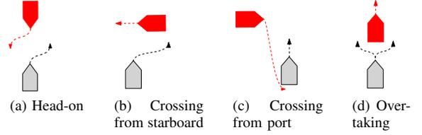
Fig. 2: COLREGs scenarios and actions for two power-driven vessels. The scenarios are described from the gray vessel's perspective.
