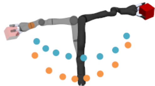
Fig. 8: The end effector path of sad trajectories generated with the neural network (blue) cost and the featurized (orange) cost, for the carry task.
