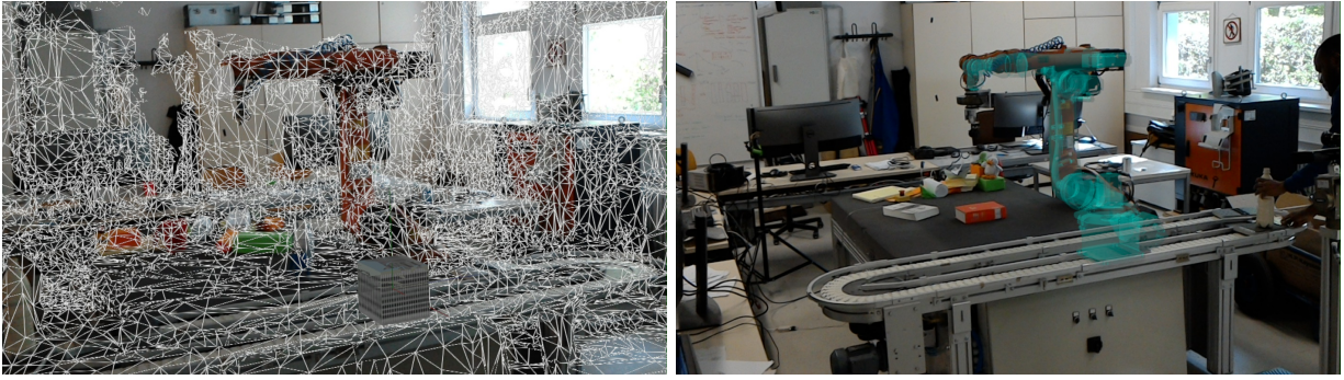
Fig. 5. The results of the referencing algorithm; (left) The HoloLens spatial mesh and the seed hologram positioned by the user; (right) The hologram overlaid on the real robot
