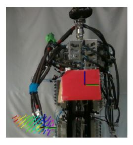
Fig. 1. 10 DoF musculoskeletal robot arm actuated by 24 pneumatic artificial muscles (PAMs), with an empirically defined goal space in reference to the red marker, visualized in rviz.
