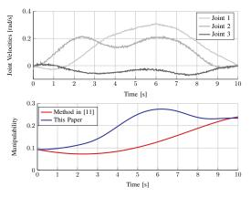
Fig. 8: Top: Velocities of the three largest UR-10 joints using our method. Bottom: Manipulability values compared to [11].
