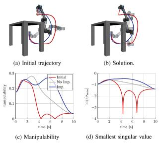
Fig. 5: Reaching a goal configuration while avoiding an obstacle. Top: Visualization, the final state is opaque. Bottom: The manipulability and smallest singular values with and without the use of interpolated states.
