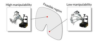
Fig. 1: Comparison of two solutions for reaching a position goal from a given near-singular starting configuration (caused by fully extending the arm initially). The right image shows a solution based purely on inverse kinematics, which maintains low manipulability throughout. The image on the left shows a trajectory generated by our method, which avoids excessive arm extension.
