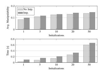
Fig. 6: Performance of our method for the task described in Section V-C with respect to the number of initial trajectories computed. Top: Average manipulability during task execution. Bottom: Solve time.
