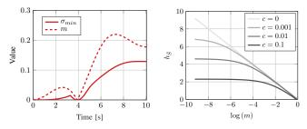
Fig. 3: Left: Comparison of the manipulability measure (dashed line) and the smallest singular value of the Jacobian throughout a trajectory. Right: Shape of the likelihood function in Eq. (10), which depends on the parameter c.
