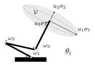
Fig. 2: Illustration of the manipulability ellipsoid of volume  $\mathcal{V}$  for a manipulator end-effector at configuration  $\boldsymbol{\theta}_i$ . Larger axis lengths indicate higher mobility.
