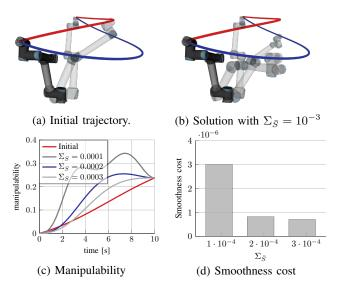
Fig. 4: Reaching a goal configuration. Top: Visualization, the final state is opaque. Bottom: The manipulability and smoothness costs for different  $\Sigma_{\bar{S}}$ .
