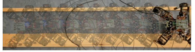
Fig. 8: Overlay of all the locations selected to place foot as the robot walks from right to left. As you can see, the robot kept a straight line along the beam and did not fall off.
