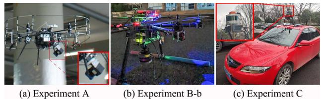
Fig. 8. Sensor configurations in experiments. (a) A MAV with a spinning 2D lidar [2] in the experiment A. (b) A MAV with a 3D lidar and onboard computer in the outdoor test in the experiment B. (c) A 3D lidar and an IMU on passenger vehicle in the experiment C.
