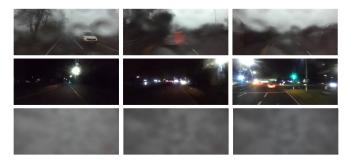
Fig. 9: Images Collected in Fog/Rain (top), Night (middle) and Snow (bottom). Images quality significantly degrades in these conditions, making it extremely challenging for vision based algorithms. Note for the snow sequence at bottom, the camera is completely occluded by the heavy snowfall.
