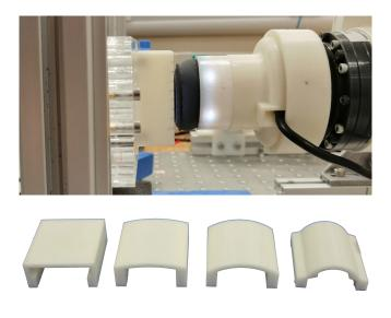
Fig. 7: Top: Flat stimulus held by the tip for real time testing. Bottom: Experiment stimuli with differing radii of curvature.
