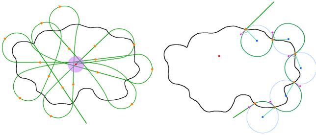
Fig. 3. Rosette (left) and Lace (right) trajectory
