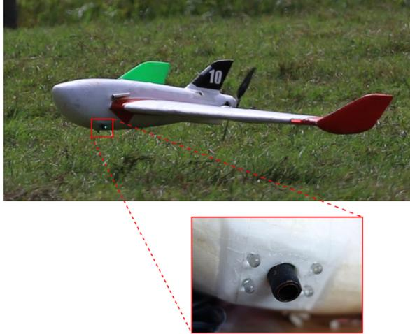
Fig. 5. X6 UAV, close-up on the cloud sensor
