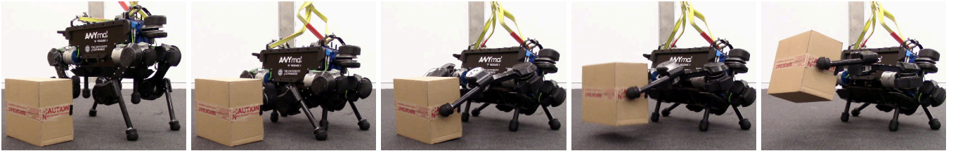
Fig. 9: The support provided by the prongs is used to free two of the legs for a manipulation task (i.e., lifting a box)
