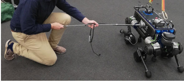
Fig. 5: The push recovery experimental setup. The robot is pushed using a stick with a force/torque sensor.
