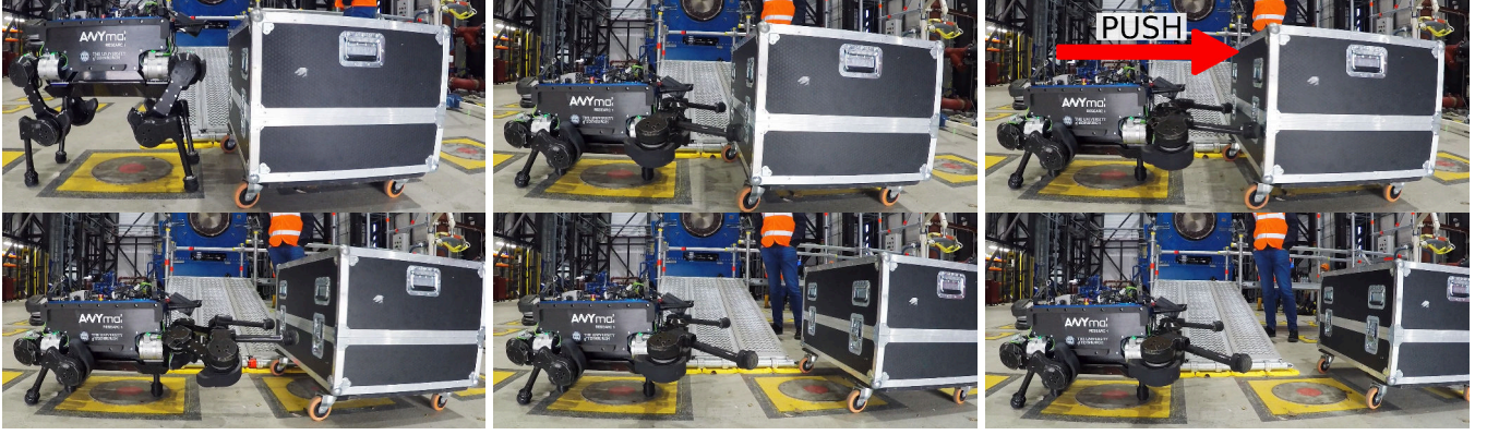
Fig. 7: The robot leaning on both prongs to push a box away. From top left: From a standing position (1), the robot lowers itself onto the prongs (2), which enables the front legs to be lifted from the ground. These front legs are used to push the box (3), which is pushed out of the way (4-6), clearing space for the robot to move into.
