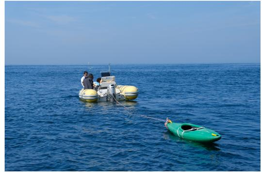
Fig. 2. Boatbot towing a magnetometer
