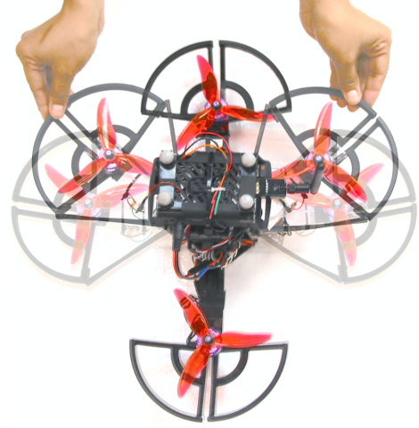
Fig. 1: The quadrotor design proposed in this paper with a passive adaptive morphology when interacting with the environment. videolink: https://youtu.be/0GEBscTuoDA
