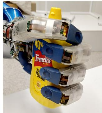
Fig. 1. A high-quality grasp planned in simulation and executed on the DLR-Hand II [7].
