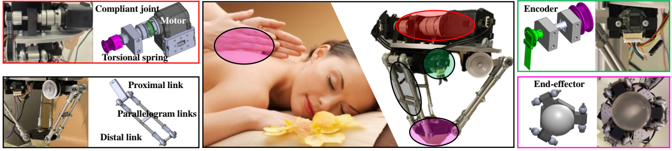
Figure 1. The design of the proposed parallel mass manipulator consisting of compliant joints, encoders, links and end-effector. A potential application scenario where the proposed massage robot can perform a tapping massage task (Middle figure).
