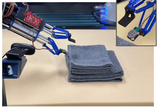
Fig. 1: We present a tactile-based cloth manipulation system. The robot utilizes a ReSkin [2] sensor attached to the lower one of its two fingertips, which is visualized in more detail in the upper right inset. We train a classifier to distinguish among grasping different numbers of cloth layers from tactile feedback (no images are provided as input). The robot then uses this classifier at test time to determine suitable grasping points for obtaining a desired number of cloth layers.
