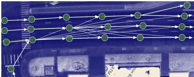
Fig. 1: The routing graph built on a lane-level map. Nodes are fixed lane waypoints, and edges are maneuvers between them (not all lane changes are shown for clarity).
