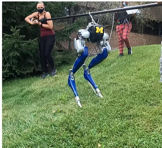
Fig. 1: Cassie Blue using a 3D-ALIP inspired MPC gait controller to walk sideways up a  $22^\circ$  incline on wet grass. Lateral walking with Cassie is much more difficult than longitudinal walking due to tight workspace constraints, which are accounted for in our formulation.
