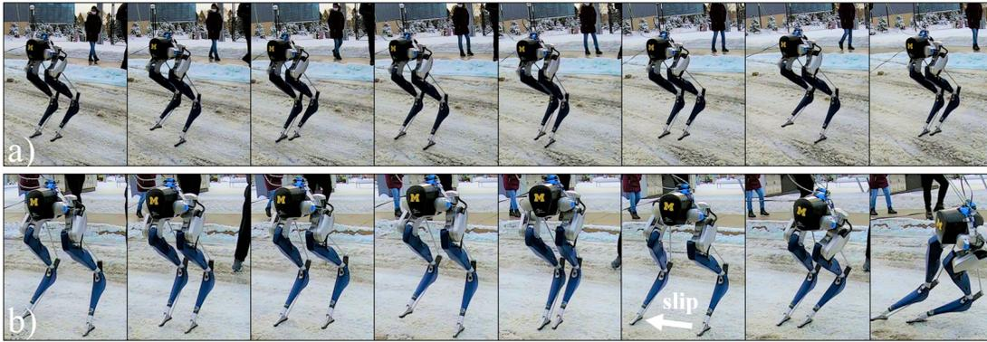
Fig. 6: Lateral walking (desired 1 m/s) on snow/ice mixture for friction coefficients (a)  $\mu = 0.6$  and (b)  $\mu = 1.0$ . The slip constraint is embedded in the intra-step dynamics of the MPC formulation. In (b) Cassie slips when the magnitude of the lateral CoM component is too large whereas in (a), the more cautious friction coefficient properly restricts the foot position, and thereby limits the robot's speed.
