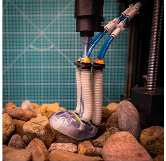
Fig. 1: Four tendon units integrated into a robotic ankle, showing compliance over rough terrain.
