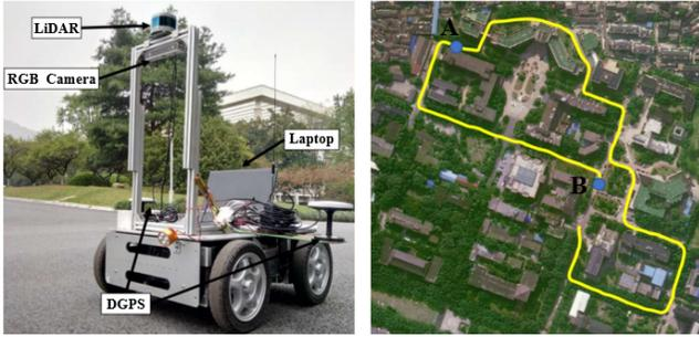
Fig. 8: The collection of the YQ dataset. The left image shows the data collection platform. The yellow line of the right image shows the trajectory of the data collection on our campus.
