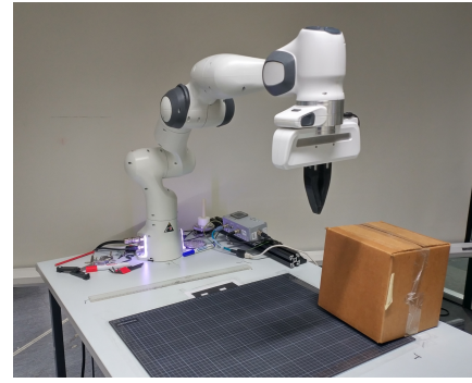
Fig. 6: The real world FindBox setup with Franka Panda.
