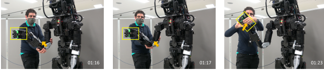
Fig. 9. Testing the dual compliance, when moving on the arm, only the null-space of the task is compliant, therefore the hand remains in the same position, but when interacting with the hand itself the admittance control is triggered and the end effector can be moved freely.
