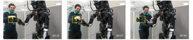
Fig. 7. Testing the control without the proposed null-space compliance, the hand position is stiff and it is difficult to move in the null-space.
