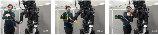
Fig. 8. Testing the control with null-space compliance. The hand position is still stiff but now it is much easier to move the robot in the null space of this task (2 DoF tested.)
