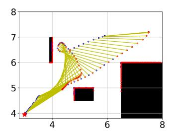
Figure 5: Trajectory snapshot of the rod with a switching leader-follower role allotment and learning obstacles from the follower inputs. The task succeeds.
