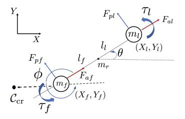
Figure 2: Model of the joint system. The leader and the follower are point masses connected by the rigid rod. The follower reacts to a *critical obstacle*  $C_{cr}$ , as defined in Section 3.1.
