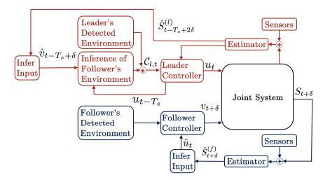
Figure 1: Block diagram of the joint system with leader follower controllers.
