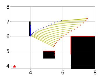
Figure 4: Trajectory snapshot of the rod with a fixed leader-follower role allotment and learning obstacles from the follower inputs. The task still fails.
