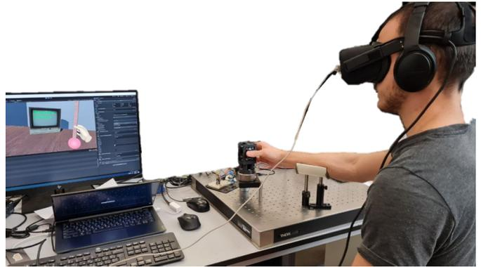
Fig. 1. Experimental procedure: a user wearing VR goggles is using the haptic device to perform the task (seen on the screen).
