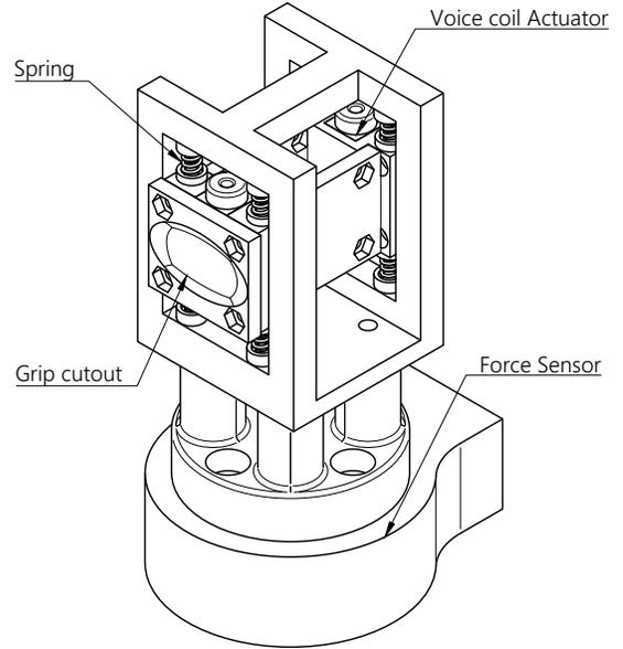
Fig. 3. Wireframe view of device in full assemble
